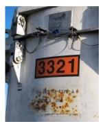
Can rust be part of or obscure the DOT specification and/or manufacturer markings? What are the package and manufacturer marking visibility requirements in both 49 CFR 172.304 and 178.3? The rust seems to be only in the area where the magnetic cover was placed over these manufacturer markings. Who is responsible to ensure the manufacturer markings meet the visibility requirements, the shipper and/or the manufacturer?
